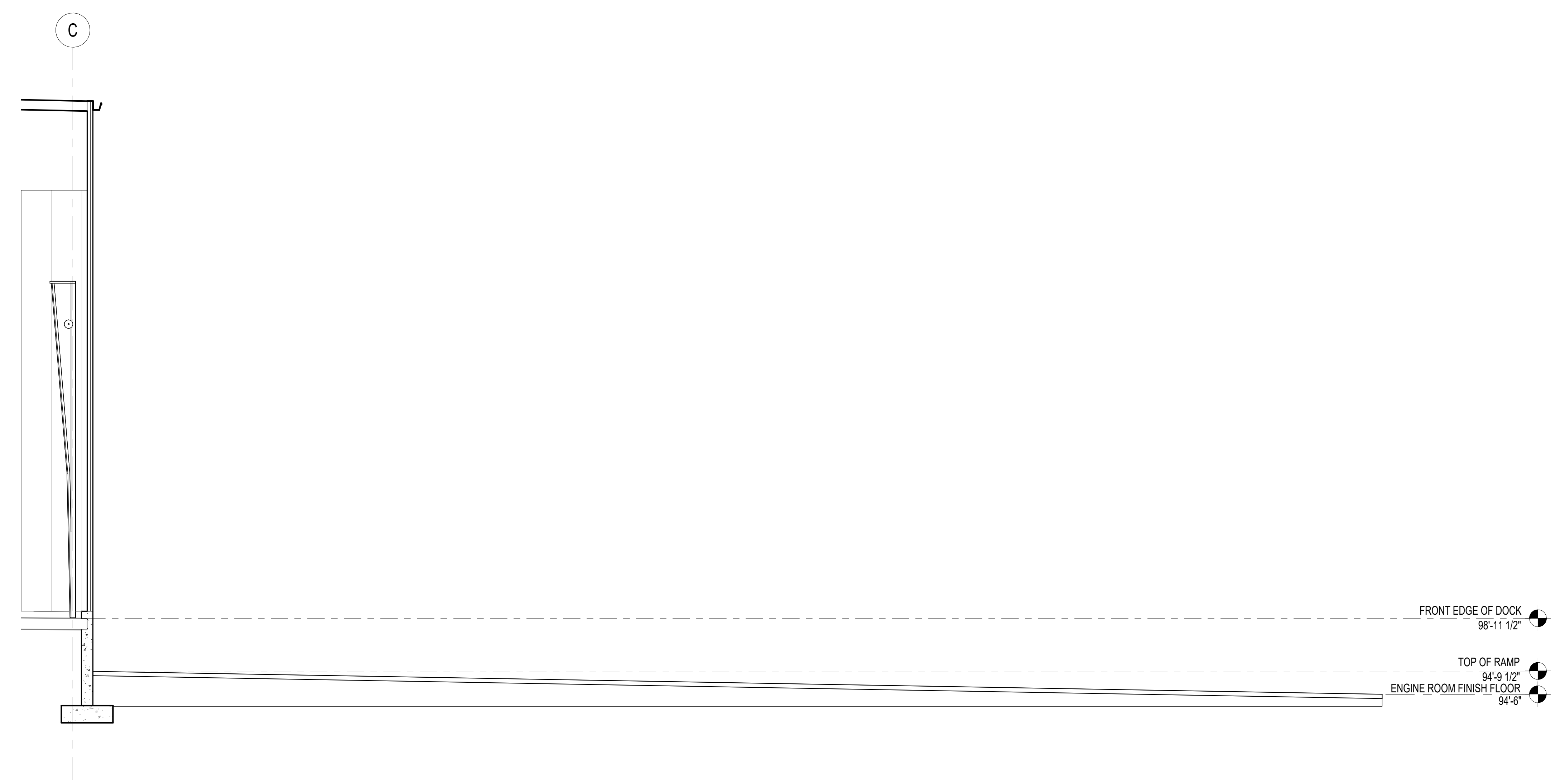
5B DOCK RAMP SECTION SCALE: 1/4" = 1'-0"
