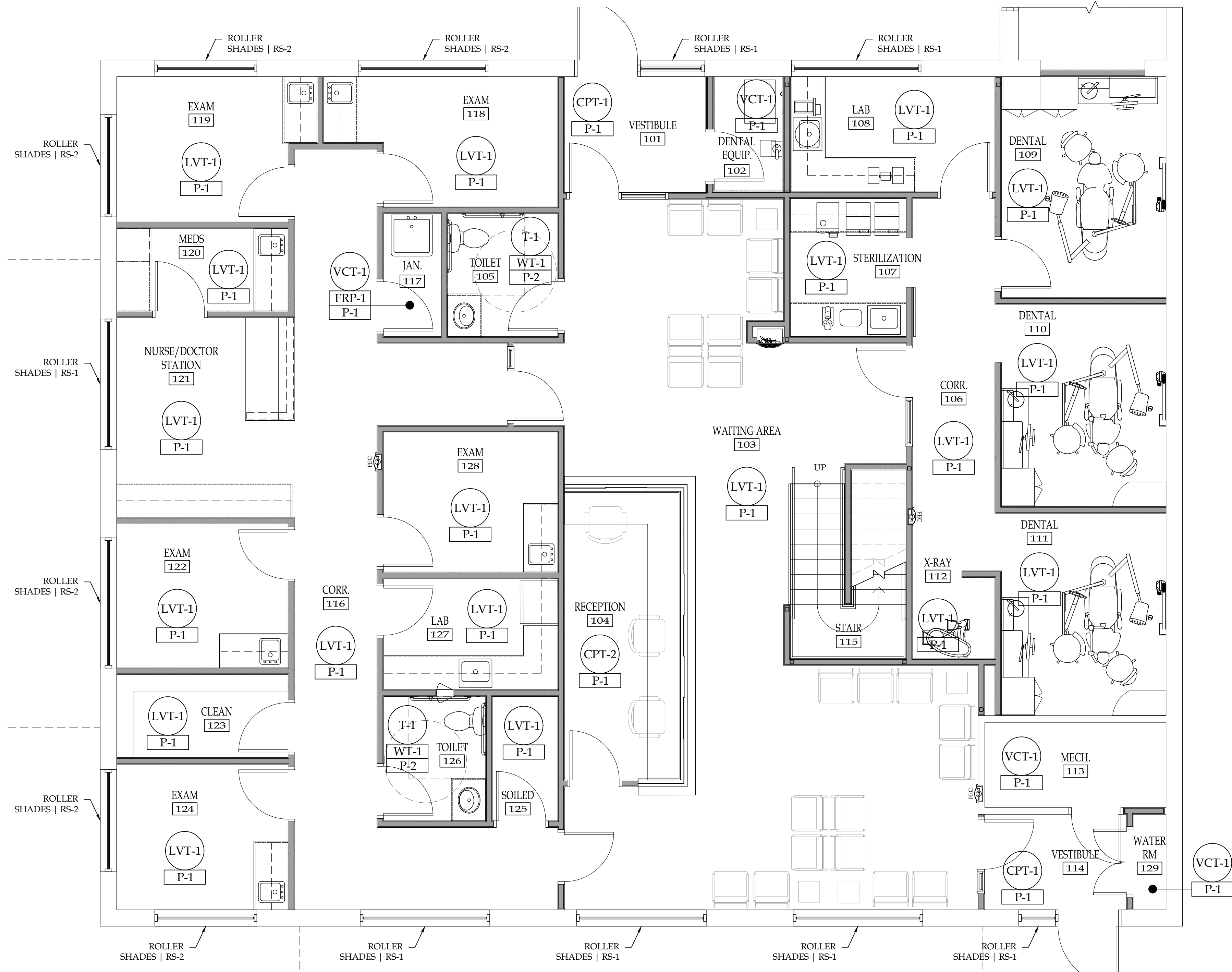
A2 FIRST FLOOR FINISH PLAN 1/4"=1'-0"
