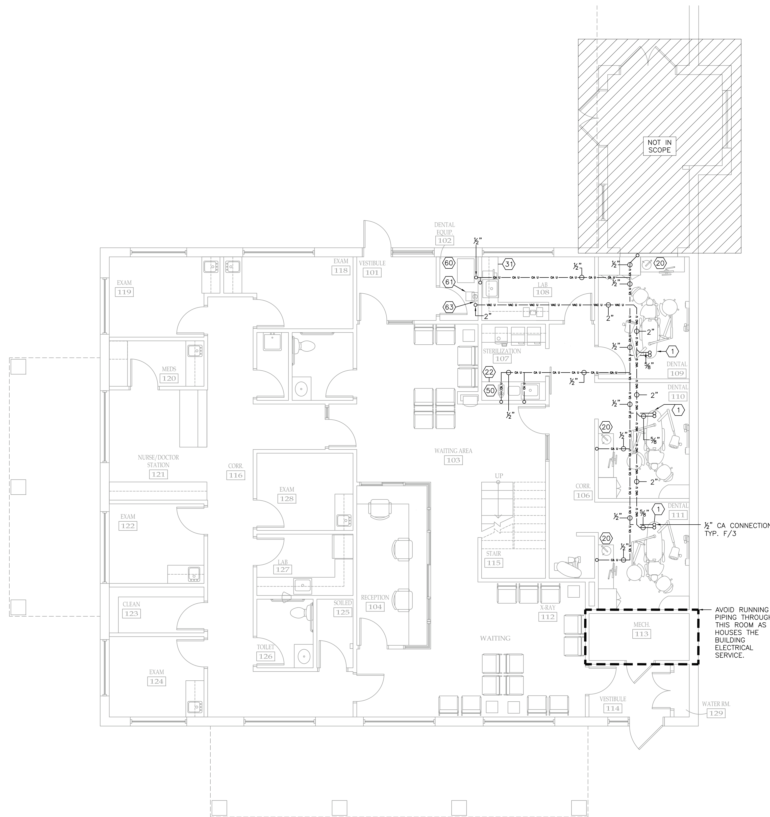
1 VACUUM + COMPRESSED AIR - 1ST FLOOR PLAN P-6 SCALE: 3/16" = 1'-0"
